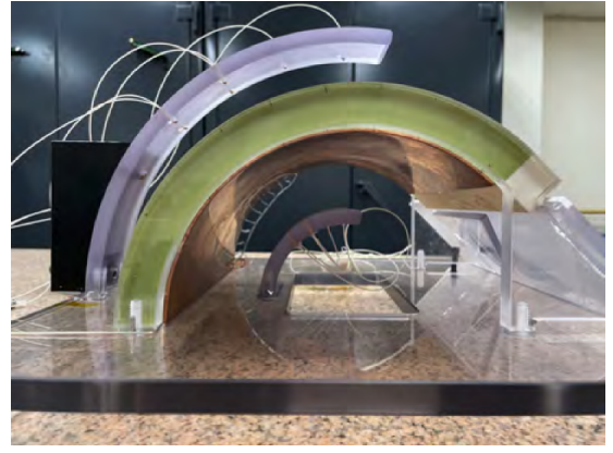
(b) HE arc assembly with copper confining wall, PDV probes (Figure 1 of [3])
