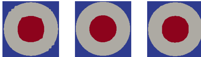
FIGURE 2: Material partition for linear advection of a three-material concentric configuration after one period. Left: Employing only the central stencil of Figure 1. Center: Employing all the candidate stencils of Figure 1. Right: Optimization via the LVIRA algorithm [1].
